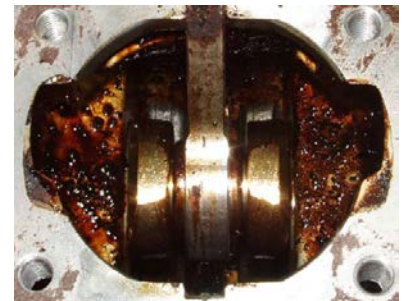
Varnish also inside crankcase
