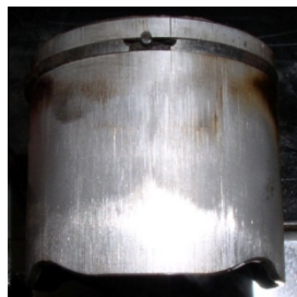
High piston intake wear
