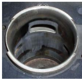
Cylinder worn below plating
