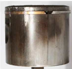
Intake side heat discoloration
